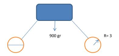
V= Volume of floatsR= Radio of floatsL = Length of floats $\rho$  = Density of water (1 g/cm ^ 3)B= BuoyancyW = Weight (900 g)I needB > Weight \* 2B = 2 floats \*  $\pi$  \* R ^ 2 \* L \*  $\rho$  = 2 \*  $\pi$  \* 3 (cm) ^ 2 \* 32 (cm)\* 1 (g/ cm ^ 3) = 1800 g
