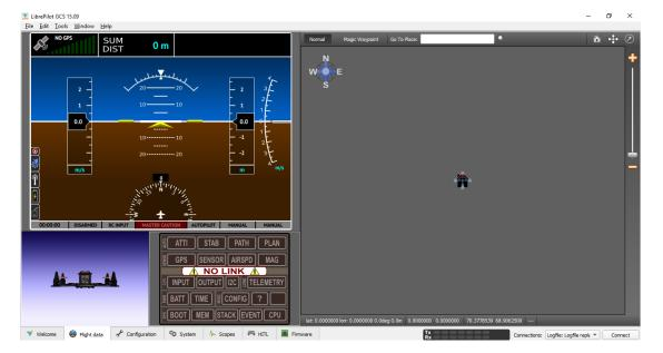
The screen show you the Flight Data panel. Now the drone is not connected. Since you combine drone, the panel show you the movement of drone and the status of components.
