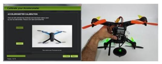
Place the drone tilting or 180 forward as shown in the picture below and press "Continue".
