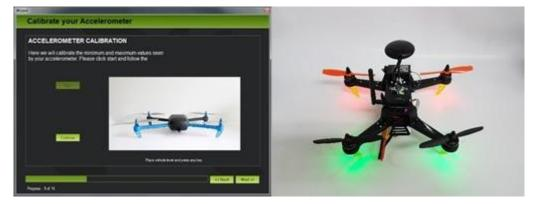
o Place the drone turned left 90 degrees as shown in the picture below and press "Continue".
