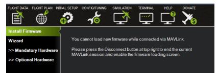
• As shown in the picture, it requests disconnection via MAVLink of the APM for upgrade. Click "DISCONNECT" on the top right of the screen.
