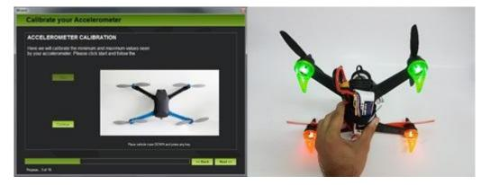
Place the drone or tilting 90 degrees backwards as shown in the picture below and press "Continue".
